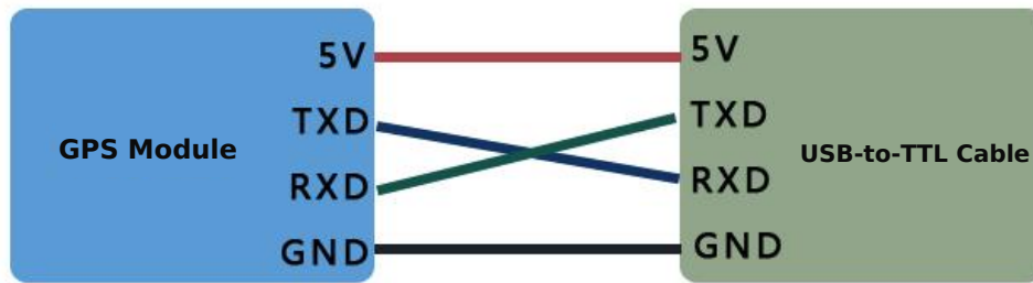
GPS Module and USB-to-TTL Cable Wiring Diagram
